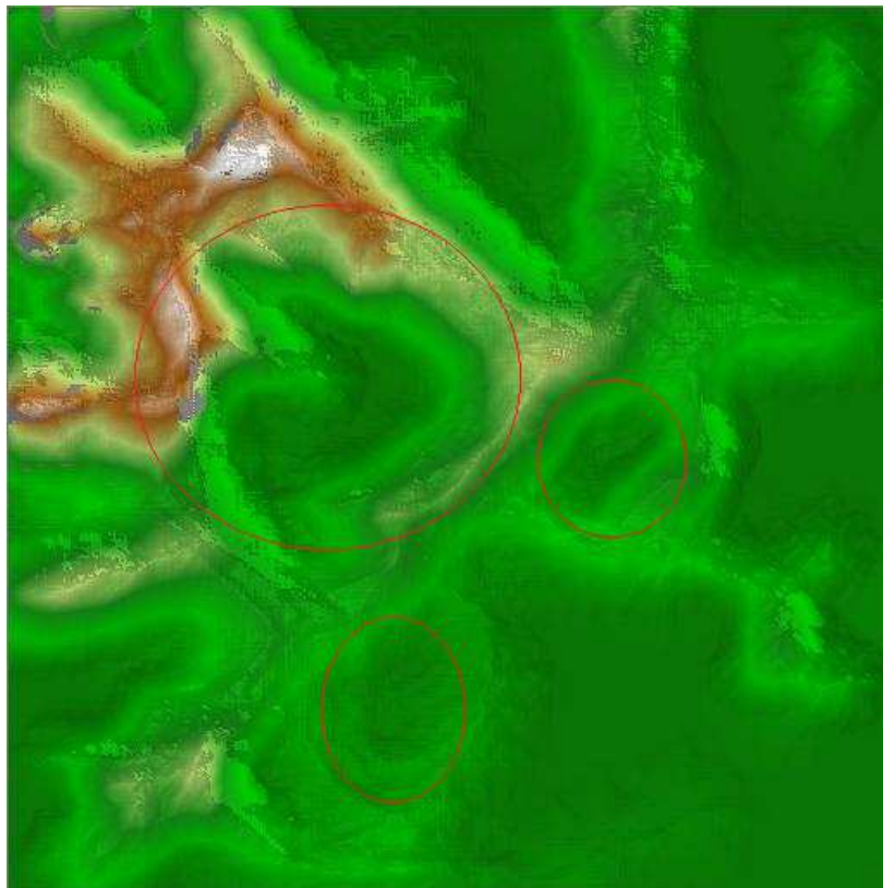
Fig.1 A terrain shape with enclosed basins.
